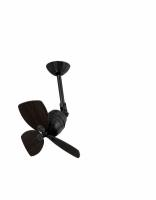
Ceiling fan suitable for rooms up to 13m2. Motor made from steel and blades from plywood .The color of blades are walnut, no reversibles. Operated by wall control,(included) setted up with 4 dimmable speeds 327 - 369 - 495 - 515 rpm which correspond to the following consumptions of 18,8 - 21,7 - 34,2 - 36,9w Airflow: 58,11 m3 min / 2052 CFM. VEDRA is suitable for inclining roof.
